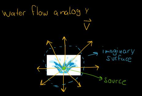
$\overrightarrow{V}$  = velocity vector field We can figure out the rate at which water is produced at the source by counting the lines that cross an imaginary surface
