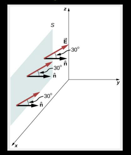
Calculate flux through <u>open</u> Surface S of area  $A = 6m^2$  located in xz - planedue to <u>uniform</u>  $\vec{E}$  with  $|\vec{E}| = 10 \text{ N/C}$ ( $\vec{E}$  makes on angle  $\dot{\Theta} = 30^\circ$  with xz - plane)
