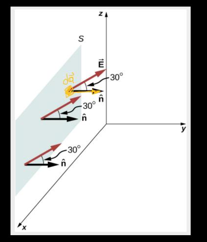
Calculate flux through <u>open</u> Surface S of area  $A = 6m^2$  located in xz - planedue to <u>uniform</u>  $\vec{E}$  with  $|\vec{E}| = 10 \text{ N/C}$ ( $\vec{E}$  makes on angle  $\vec{D} = 30^\circ$  with xz - plane)
